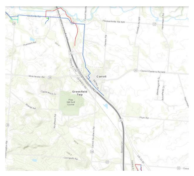
Greenfield Lift station will be located around Coonpath Road between Business Route 33 and US 33 bypass. The force main will run to the gravity sewer north of Pleasantville Road.
