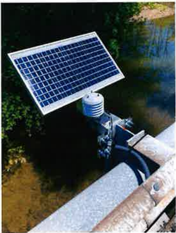
Walnut Creek got a new USGS LoCas stream gauge on Sycamore Creek at St Rt 256 for community awareness of its function and health over the next 5 years. Flow can be monitored online.
