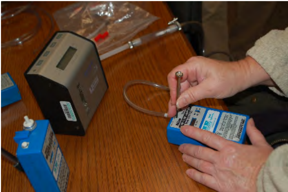
A-2. Calibration of Gilian low flow sampling pump at AA-2 using DryCal flow meter and naphthalene “calibration tube” (November 4, 2014).
