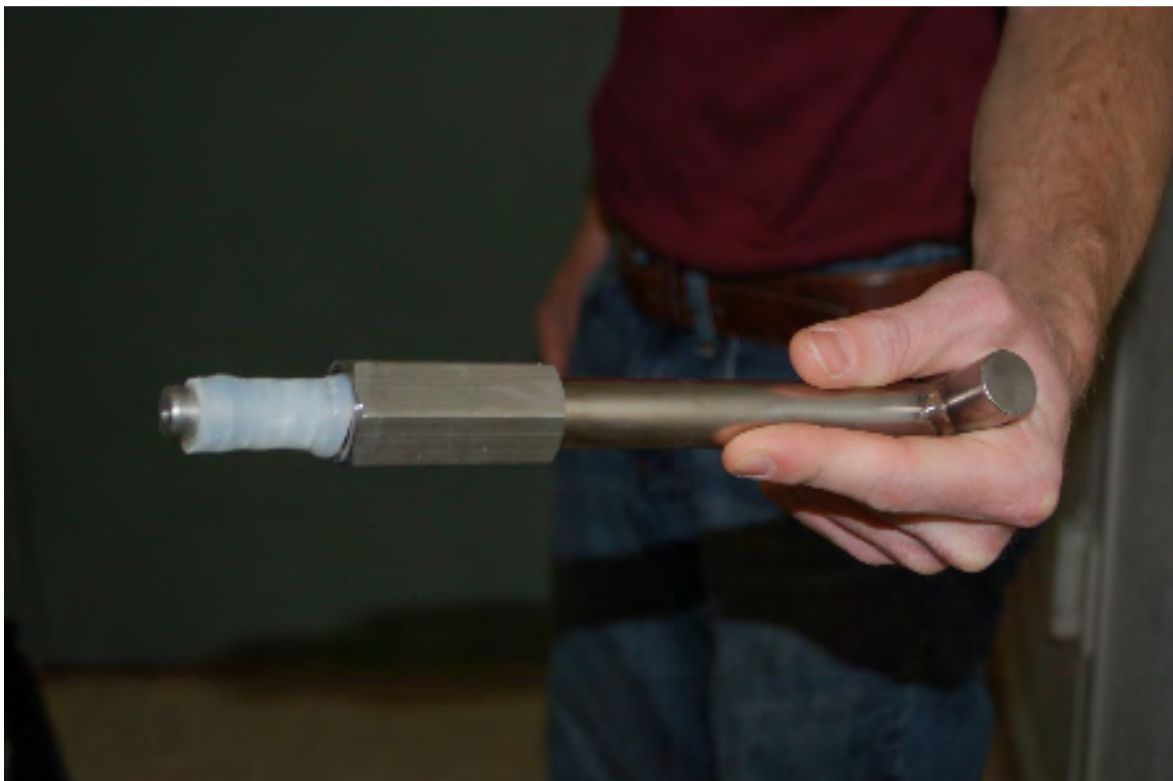
C-4. Sub-slab Vapor Pin™ assembly removed from the floor slab.
