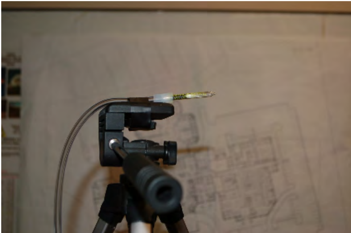
B-4. Close up of mercury tube on top of tripod during ambient air sampling at AA-2 (November 5, 2014).
