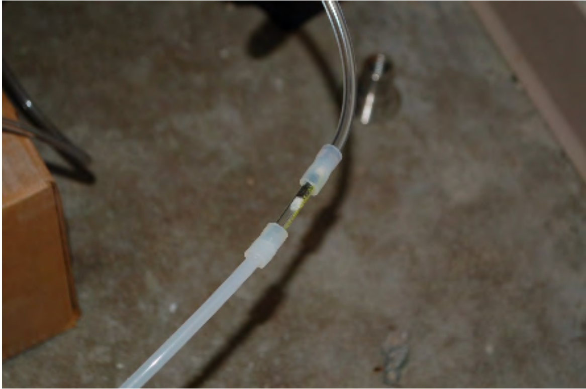
B-1. Close-up of mercury tube connected to sub-slab vapor pin (Teflon tubing) and Gilian Dual Mode Low Flow Sampler (Tygon tubing) with silicon sleeves (November 5, 2014).
