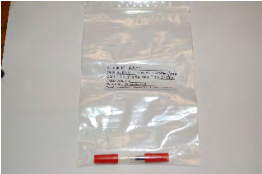
B-6. Mercury tube after sample collection with tight-fitting caps, placed in plastic bag and labelled for shipment to laboratory for analysis (November 5, 2014).
