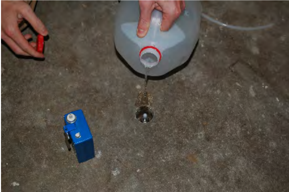
A-1. Integrity testing of sub-slab vapor sampling point SS-4 prior to sampling (November 4, 2014).
