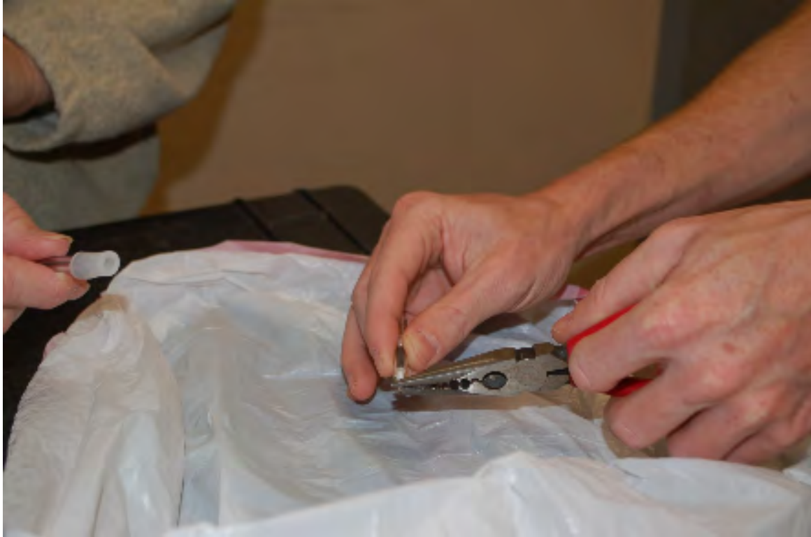
B-3. Breaking ends of mercury tube with needle nose pliers prior to sample collection (November 5, 2014).
