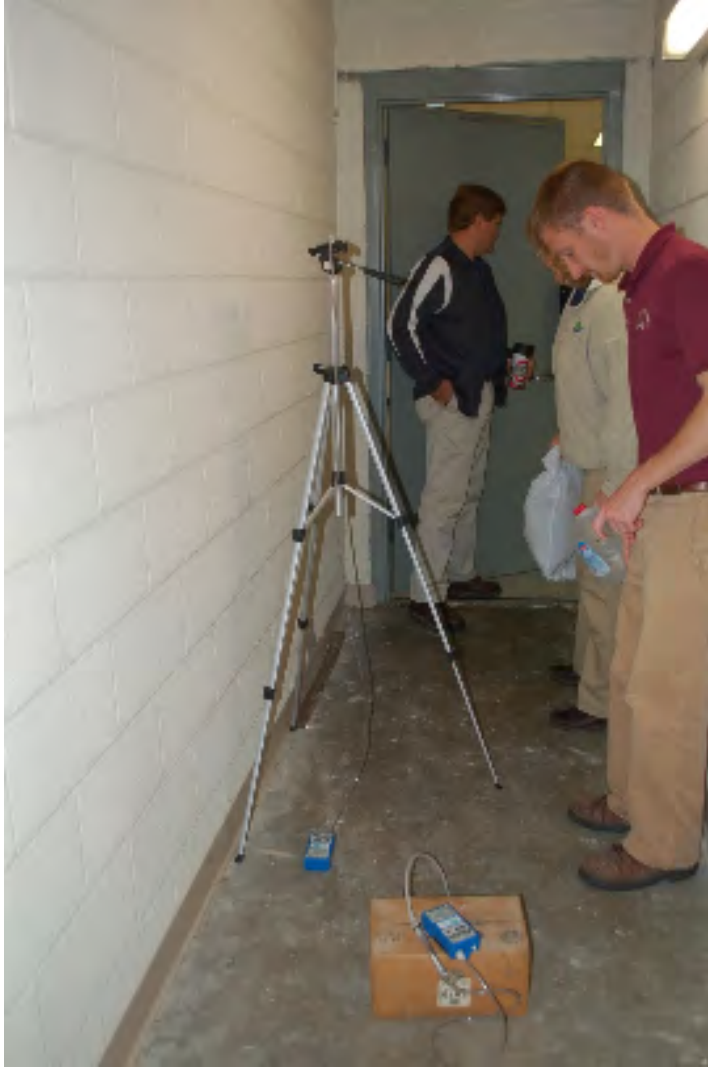
A-7. Co-located sub-slab and ambient air samples for naphthalene at SS-5 and AA-5 (November 4, 2014).
