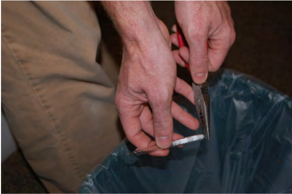
A-3. Breaking ends of naphthalene tube prior to sample collection (November 4, 2014).
