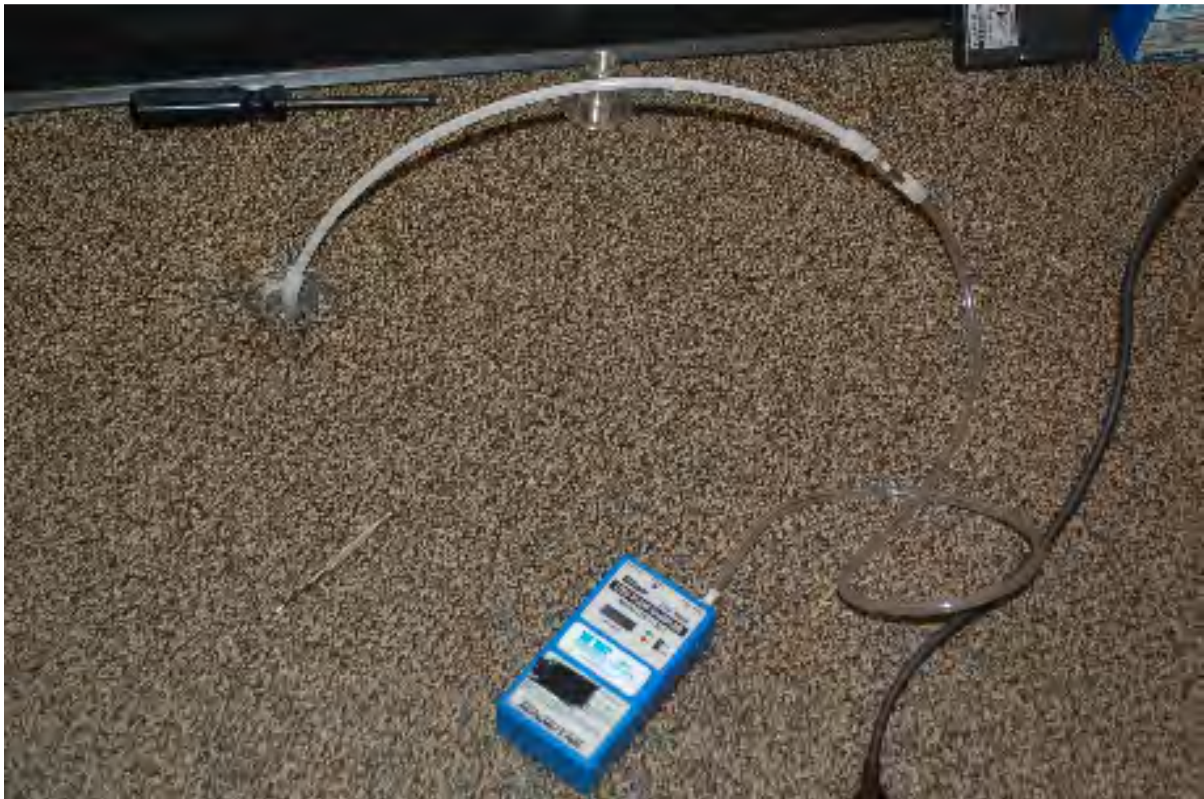
B-2. Sub-slab vapor pin sampling at SS-2 (November 5, 2014).
