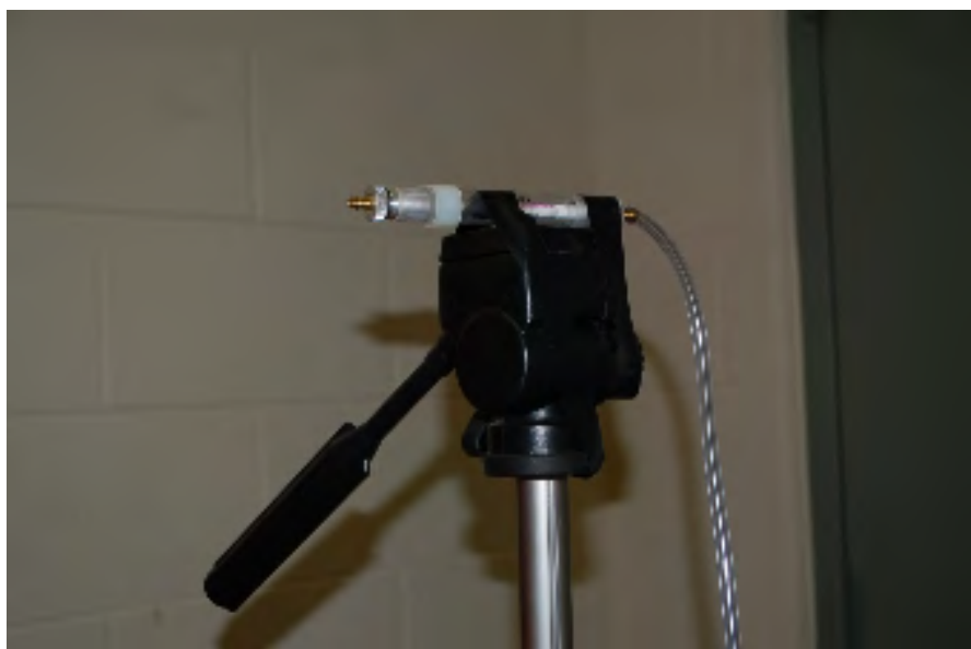
A-6. Close up of naphthalene tube in Gilian universal holder system (November 4, 2014).
