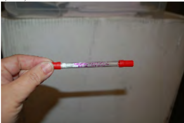
A-8. Naphthalene tube after sample collected with tight end caps prior to placing in plastic bag for labelling and shipping to laboratory (November 4, 2014).
