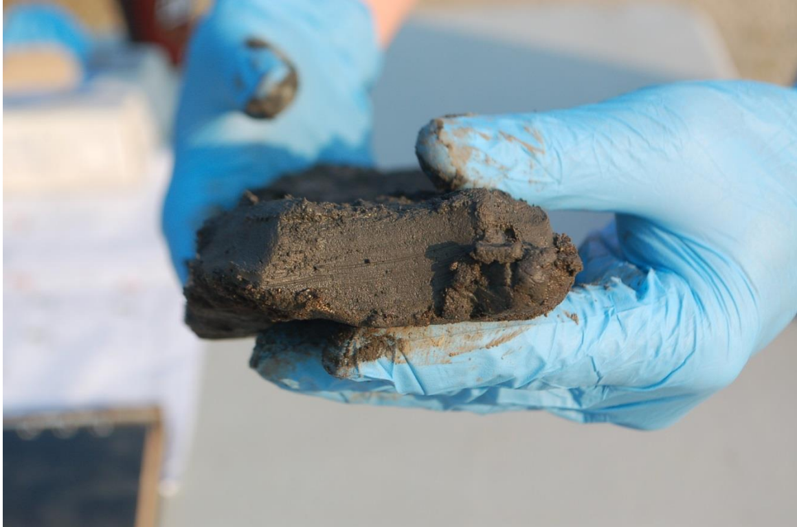
Figure B-5. Example of dark organic in-situ soils underlying the fill in some locations (September 2, 2015).
