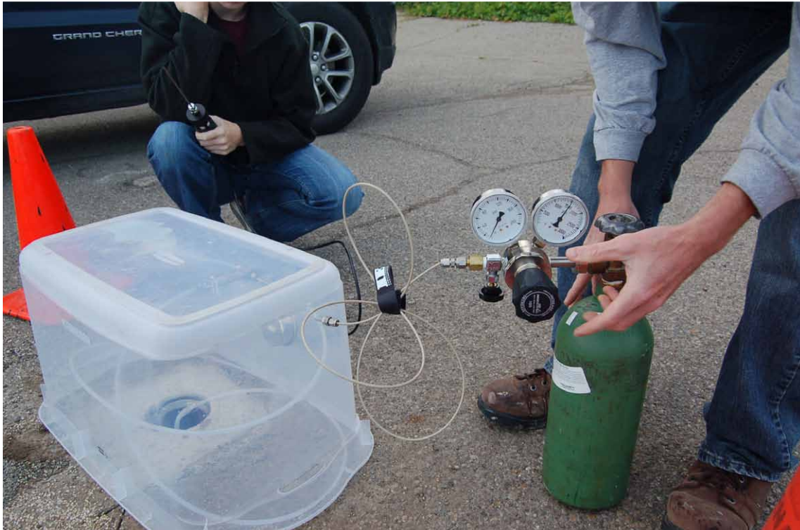
D-2. Shroud in place over subsurface soil gas probe and helium ready for flooding of shroud (July 24, 2014).
