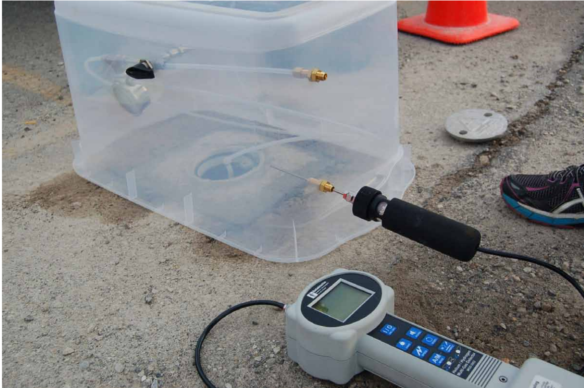
D-3. Inserting portable handheld gas detection meter to confirm presence of helium in shroud prior to pumping from the subsurface soil gas probe (July 24, 2014).
