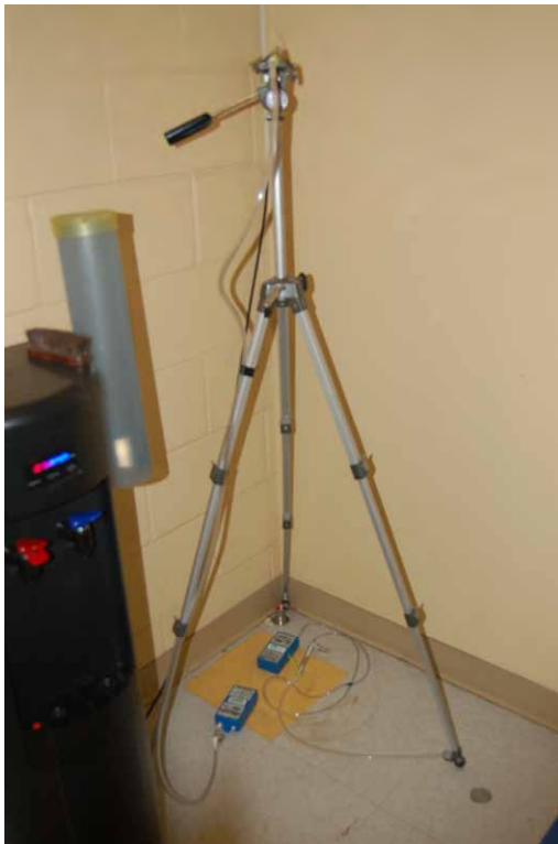
G-4. Simultaneous collection of sub-slab vapor and indoor air naphthalene samples at SS-1 and AA-1 (August 4, 2014).
