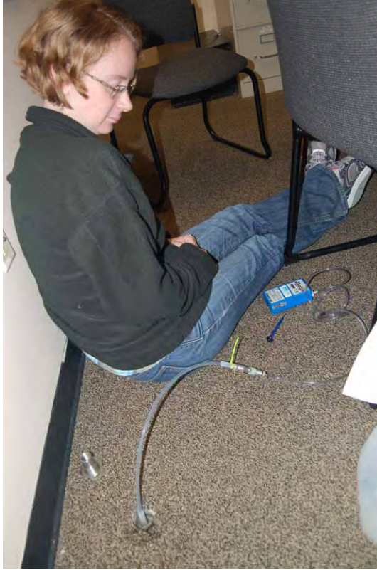
G-7. Collection of sub-slab sample for mercury at SS-2 (August 5, 2014).
