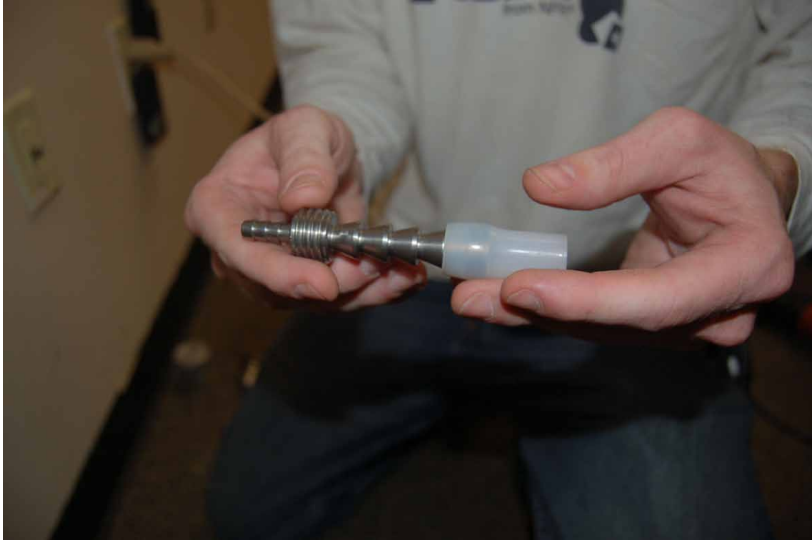
C-3. Vapor Pin™ with silicon sleeve prior to installation (July 18, 2014).
