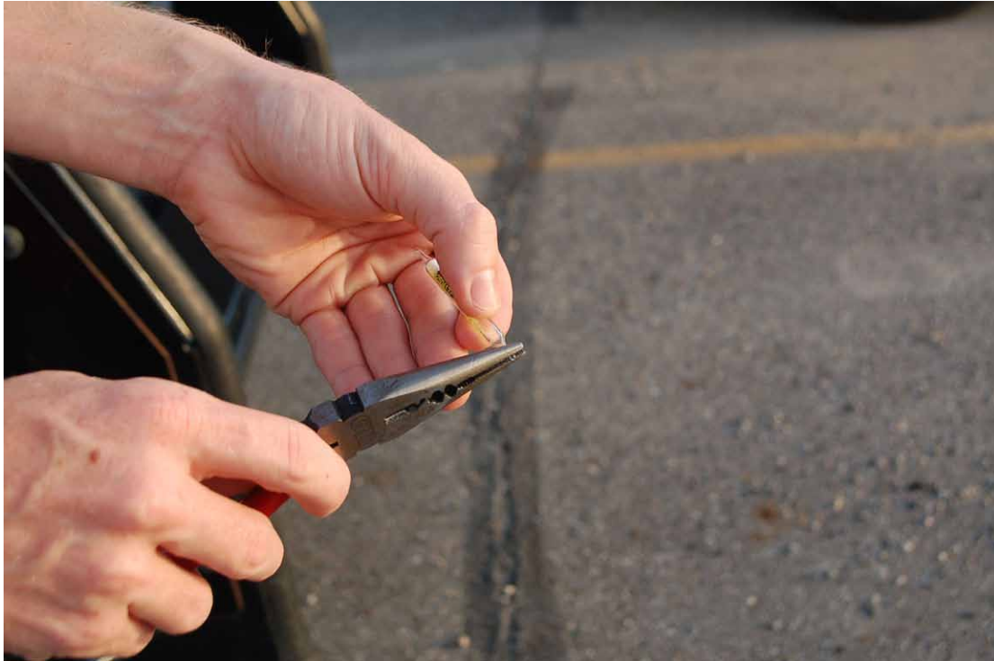
E-3. Breaking off end of tube using needle nose pliers in preparation for sample collection (September 5, 2014).
