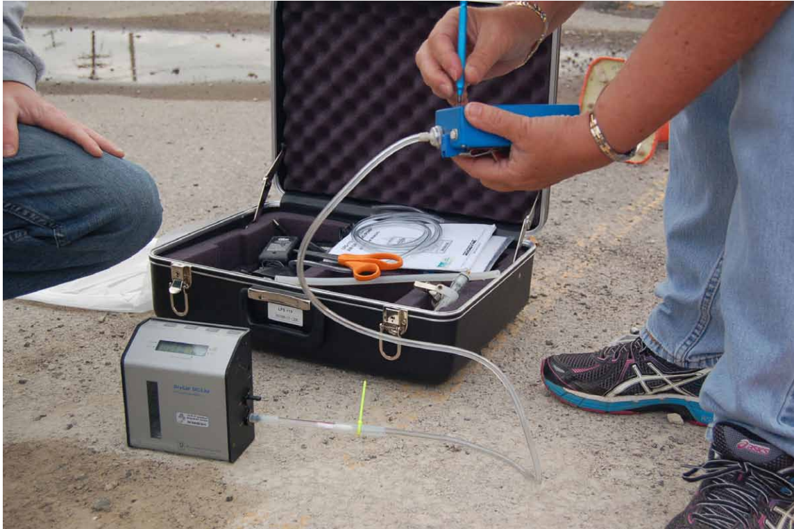
F-1. Calibration of Gilian low flow sampling pump using DryCal flow meter and naphthalene “calibration tube” (July 24, 2014).
