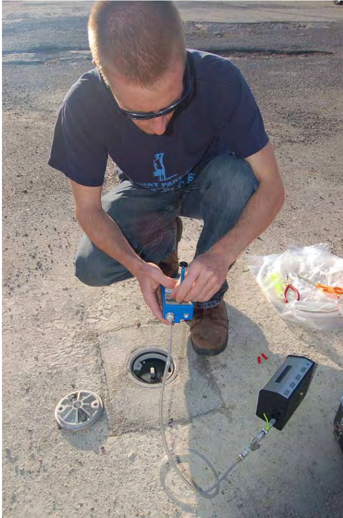
E-1. Calibration of Gilian low flow sampling pump using DryCal flow meter and mercury “calibration tube” (July 25, 2014).
