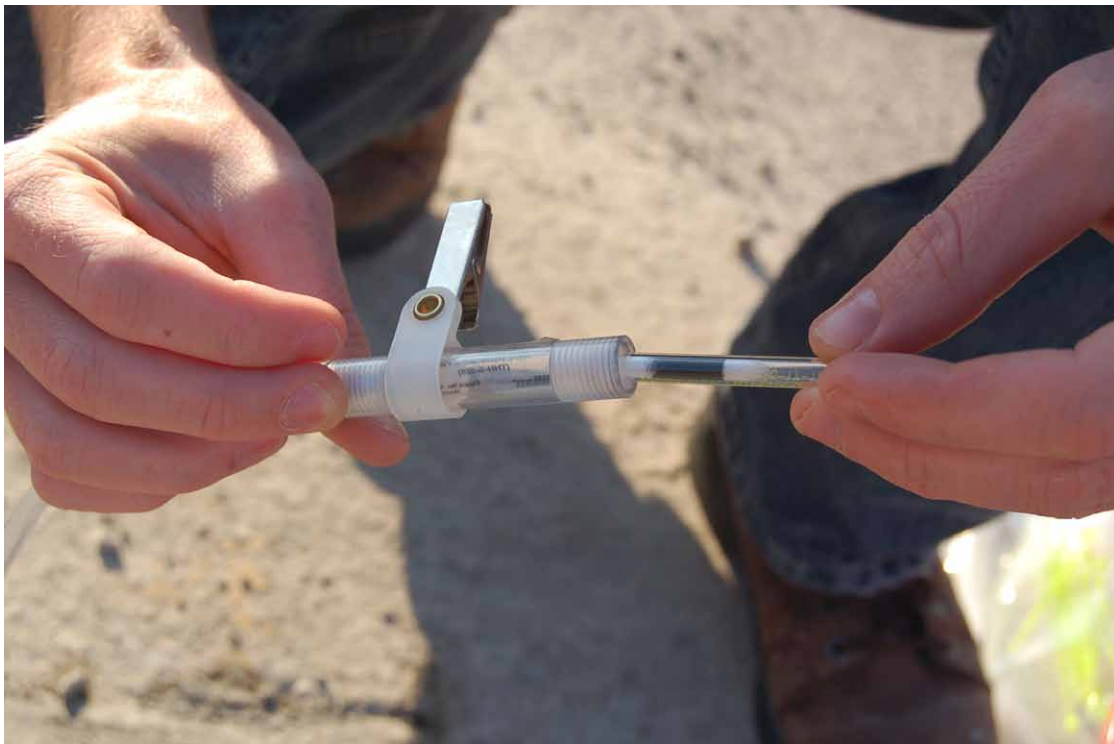
E-4. Placement of new mercury tube in Gilian tube holder (July 25, 2014).
