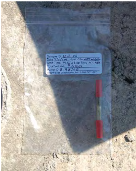
E-6. Mercury sample after collection with tight fitting caps and label ready for shipment to the laboratory (July 25, 2014).
