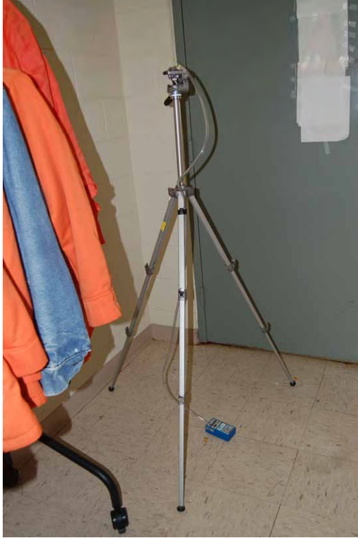
G-3. Collection of naphthalene indoor air sample at AA-4 (August 4, 2014).
