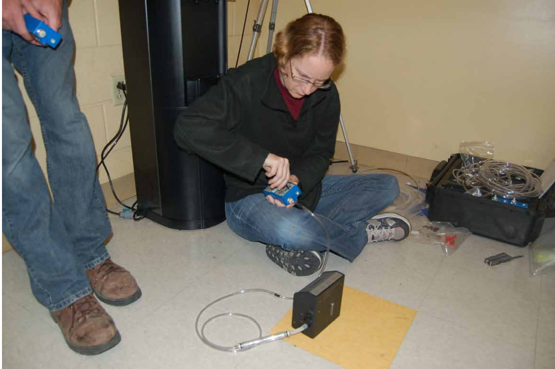
G-1. Calibration of Gilian low flow sampling pump at SS-1 using DryCal flow meter and naphthalene “calibration tube” (August 4, 2014).
