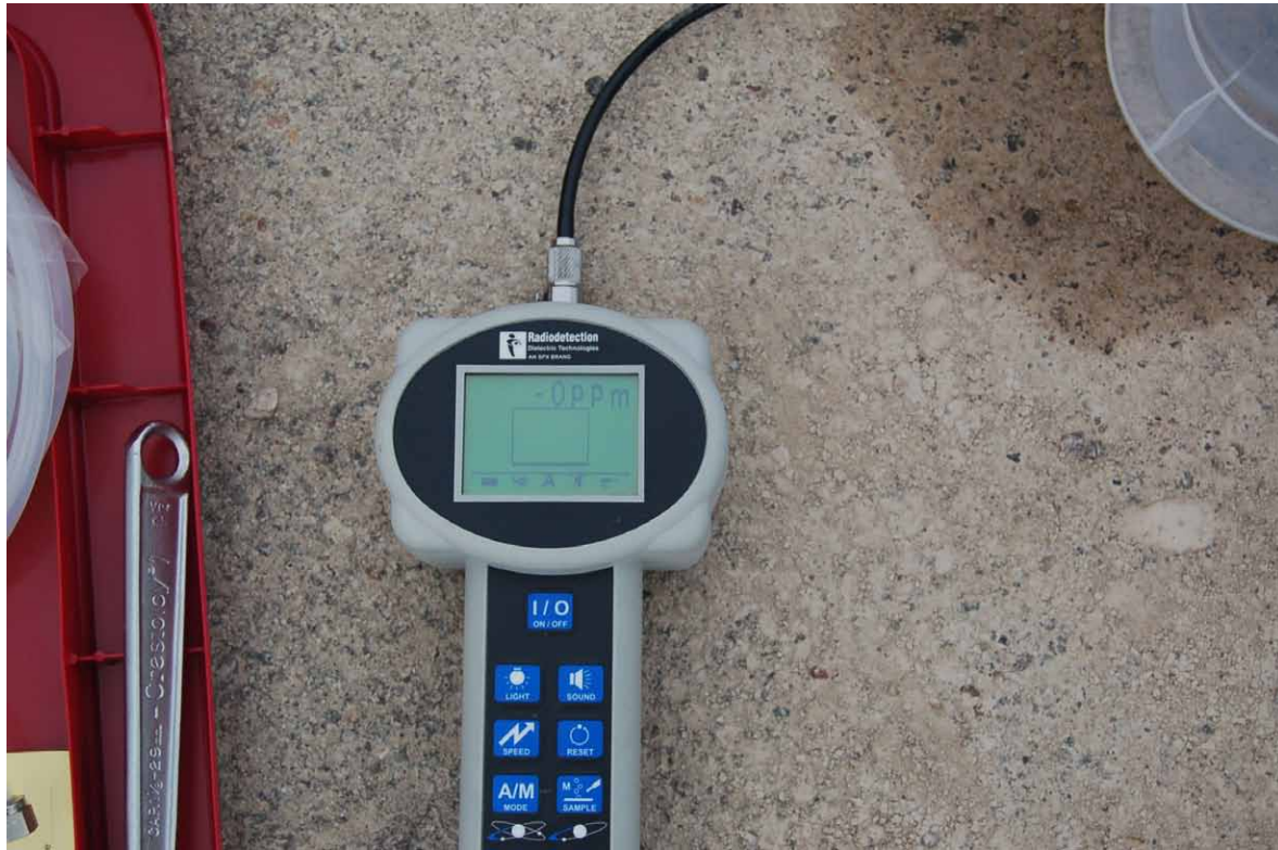
D-5. MGD-2002 portable handheld gas detection meter showing 0 ppm helium during a subsurface soil gas probe leak detection test (July 24, 2014).
