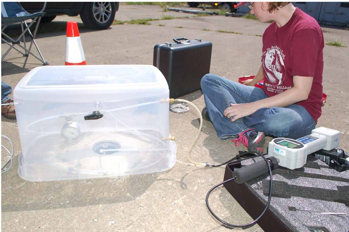
D-4. Measuring concentration of helium in subsurface soil gas probe (September 4, 2014).
