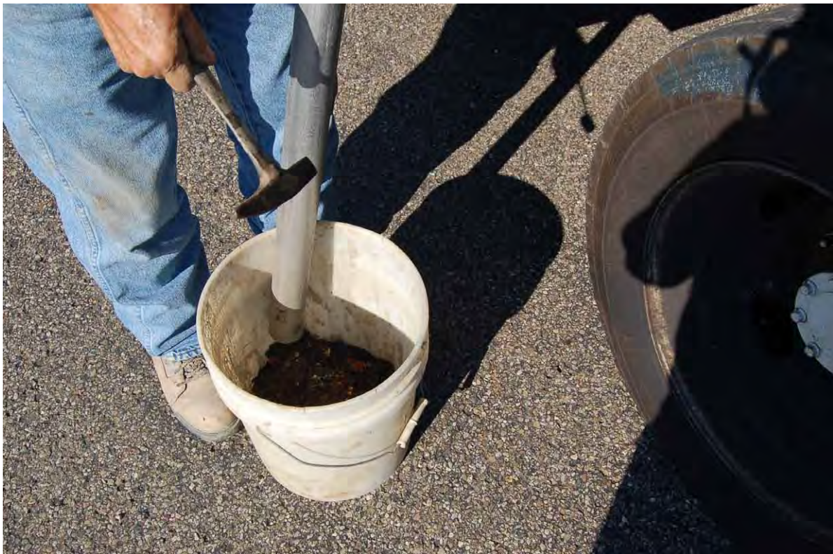
B-2. Collection of drilling cuttings in bucket before placement in 55 gallon drum (July 17, 2014).
