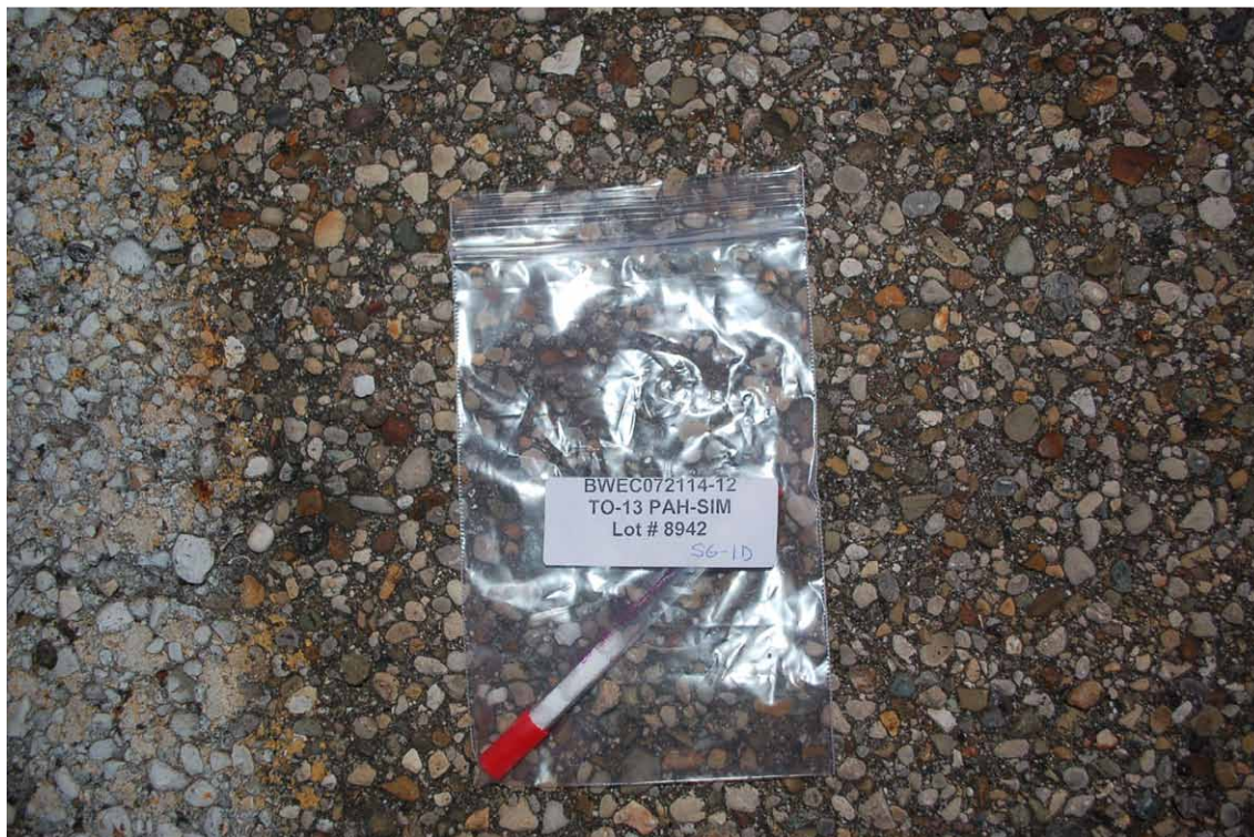
F-6. Naphthalene sample after collection with tight fitting caps and label ready for shipment to the laboratory (September 4, 2014).
