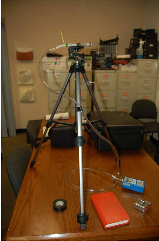
G-5. Collection of indoor air sample for naphthalene at AA-2 (August 4, 2014).
