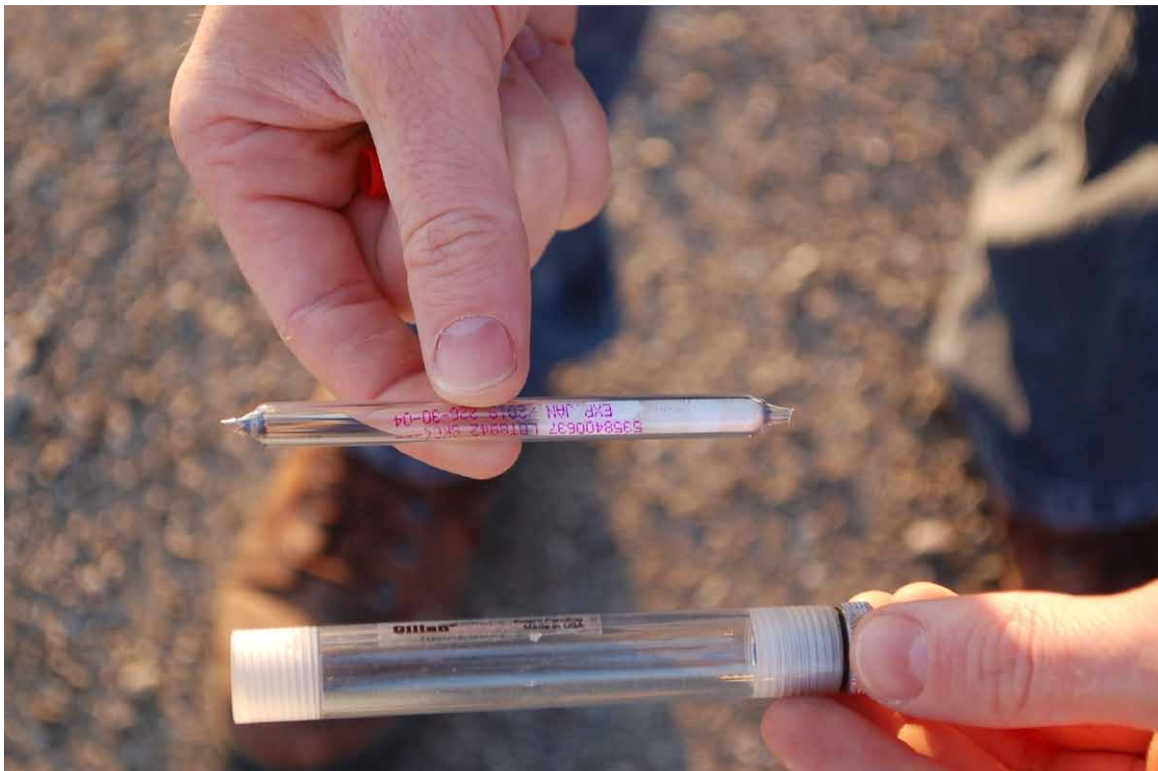
F-2. Naphthalene tube prior to placement in the Gilian Universal Tube Holder System (September 4, 2014).
