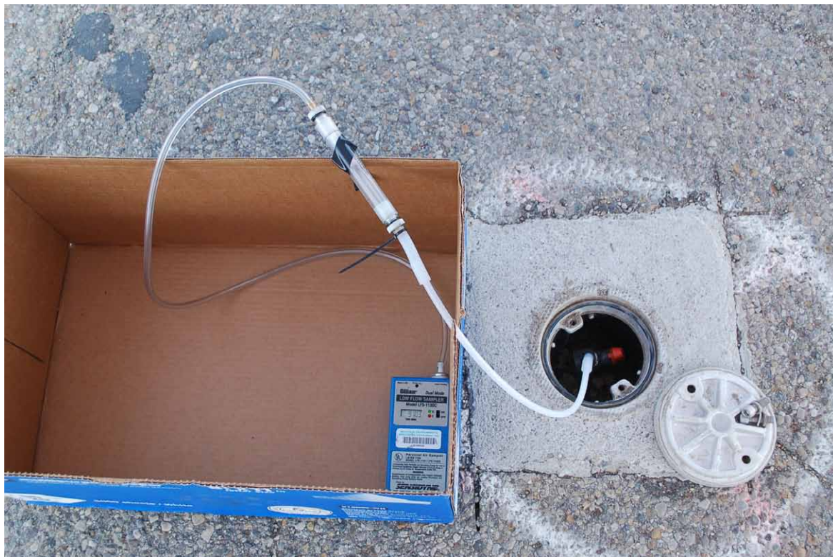
F-5. Collection of naphthalene sample using Gilian Universal Tube Holder System (September 4, 2014).
