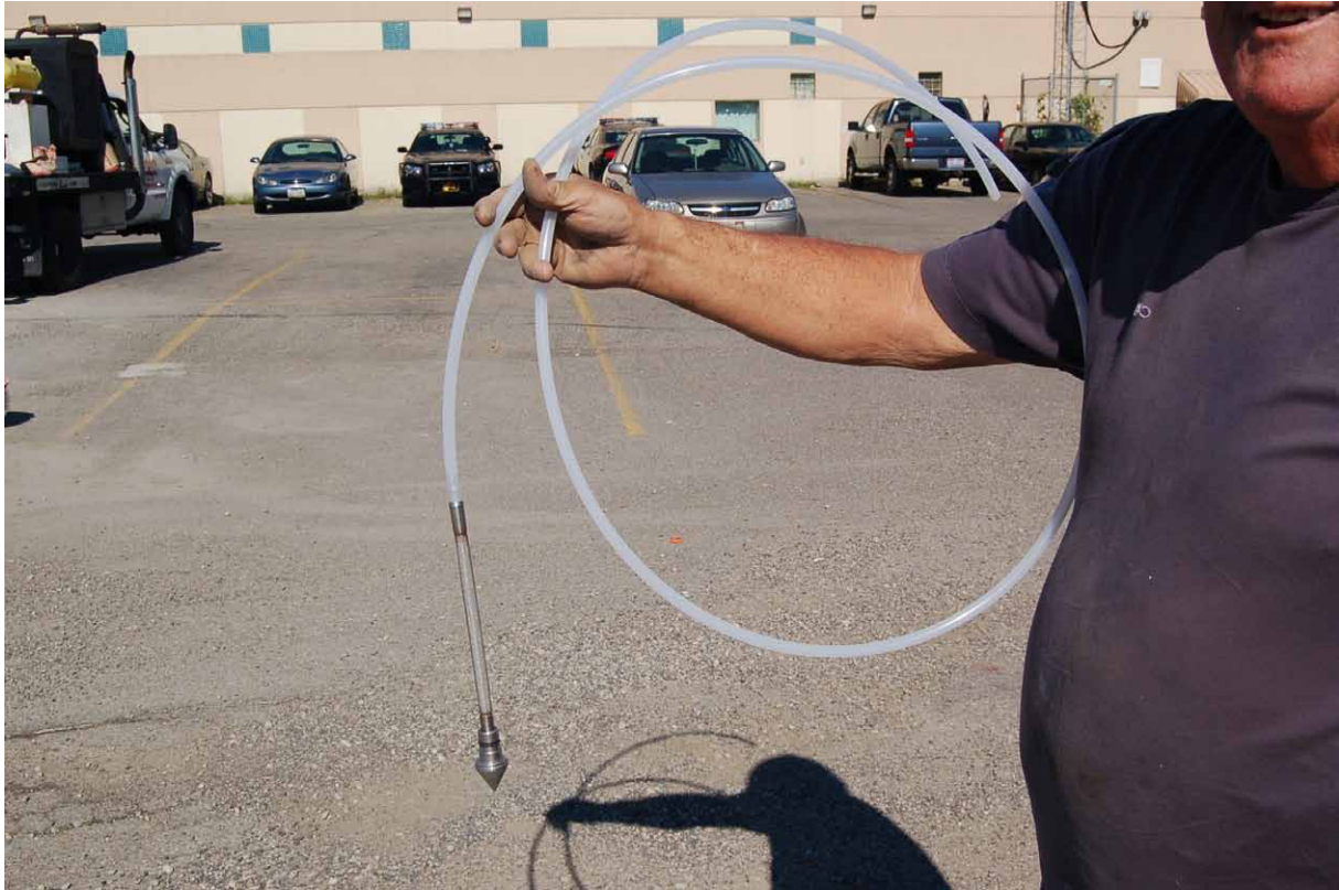
B-3. Soil vapor tip and Teflon® tubing before installation in subsurface (July 17, 2014).
